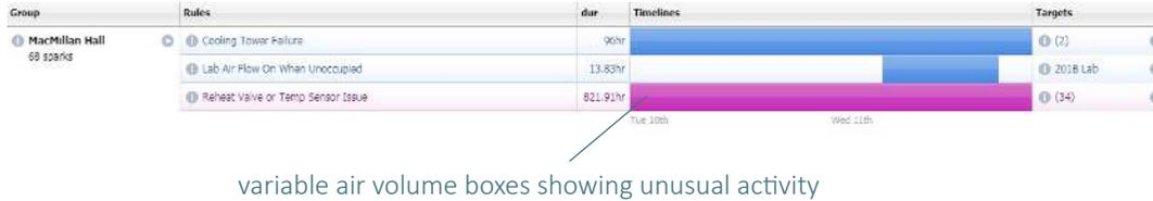
A closer look displays the problem: even though the reheat valves were closed, room temperatures were greater than the temperature of the air supplied in about 60 locations within the building.
